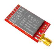
E30-TTL-100 is a 100mW wireless transceiver module with narrow-band transmission, operates at 425-450.5MHz (default: 433MHz), based on original imported RFIC SI4463/SI4438 from Silicon Labs, transparent transmission is available, WOR (ultra-low power consumption), TTL level.
