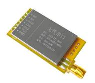
E31-TTL-500 is a 500mW wireless transceiver module with narrow-band transmission, operates at 425-450.5MHz (default: 433MHz), based on original imported RFIC AX5043 from Switzerland, transparent transmission is available, WOR (ultra-low power consumption), TTL level. The outstanding advantages of narrow-band transmission is more concentrated power densities, longer transmission distance, and better anti-interference performance.
