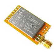
E31-TTL-50 is a 50mW wireless transceiver module with narrow-band transmission, operates at 425-450.5MHz (default: 433MHz), based on original imported RFIC AX5043 from Switzerland, transparent transmission is available, WOR (ultra-low power consumption), (ultra-low power consumption), TTL level. The outstanding advantages of narrow-band transmission is more concentrated power densities, longer transmission distance, and better anti-interference performance.
